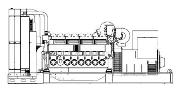
MAIN DATAContinuous power (PRP)1420.00kVAContinuous power (PRP)1136.00kWEmergency power (E.P.)1600.00kVAEmergency power (E.P.)1280.00kWVAC - HZ - cos(fi)380 - 60 - 0.8KW
