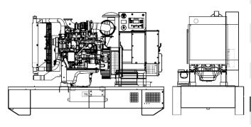
MAIN DATAContinuous power (PRP)60.00kVAContinuous power (PRP)48.00kWStand-by power (LTP)63.00kVAStand-by power (LTP)50.40kWVAC - HZ - cos(fi)400 - 50 - 0.8
