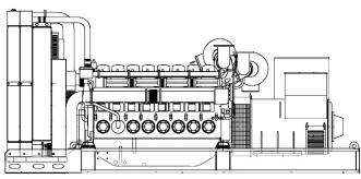
MAIN DATA Continuous power (PRP) kVA 2280.00 Continuous power (PRP) kW 1824.00 kVA Emergency power (E.P.) 2520.00 Emergency power (E.P.) 2016.00 kW 400 - 50 - 0.8 VAC - HZ - cos(fi)
