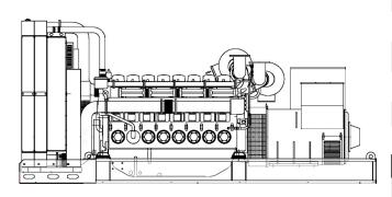
MAIN DATA Continuous power (PRP) kVA 1250.00 Continuous power (PRP) kW 1000.00 kVA Emergency power (E.P.) 1400.00 Emergency power (E.P.) 1120.00 kW 400 - 50 - 0.8 VAC - HZ - cos(fi)
