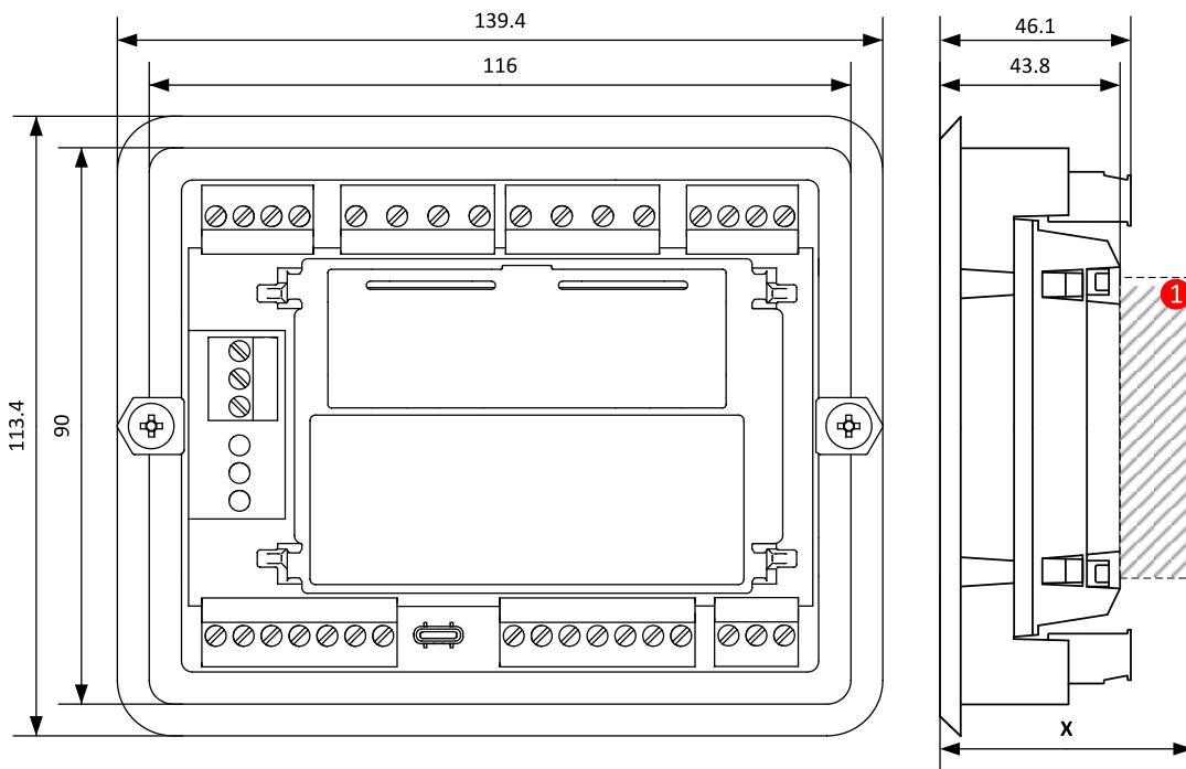
**Note:** ① The final depth "X" of the controller depends on the selected plug-in module – it can vary between 43.8 mm and 62 mm. Mind also the size of connectors and cables (e.g. in case of RS232 connector, add about 60 mm more for standard RS232 connector and cable).
